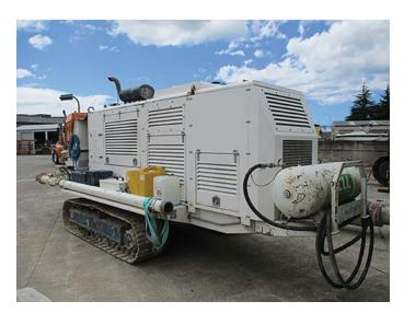
We have a variety of concrete pumps in various sizes to pump freshly mixed concrete to specific locations on the construction site.
