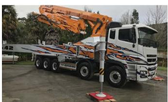
Our boom pumps are essential for pumping concrete to hard-to-reach places on large-scale construction projects.
